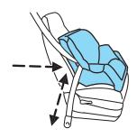
be no more than 1 inch (2.5 cm) of movement for proper installation.
